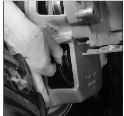
Figure 5-17: First move belt off the lower pulley.
